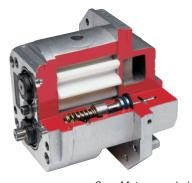
Gear Motor runs Lube Free by using close tolerance molded gears made of a high strength self lubricating composite
